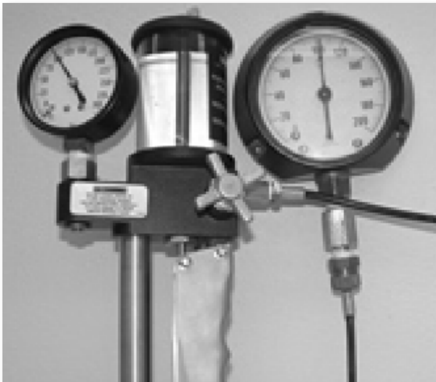
To help growers measure pesticide spray and irrigation water pressure more accurately, ARS scientists assembled an instrument for checking pressure gauge accuracy. Above, a grower's gauge (left) is screwed into a threaded port to be tested against a calibrated gauge (right).
